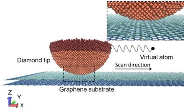
FIG. 1. Snapshot of the model system where a hemispherical diamond tip is connected to a harmonic spring which pulls it over graphene layers.
