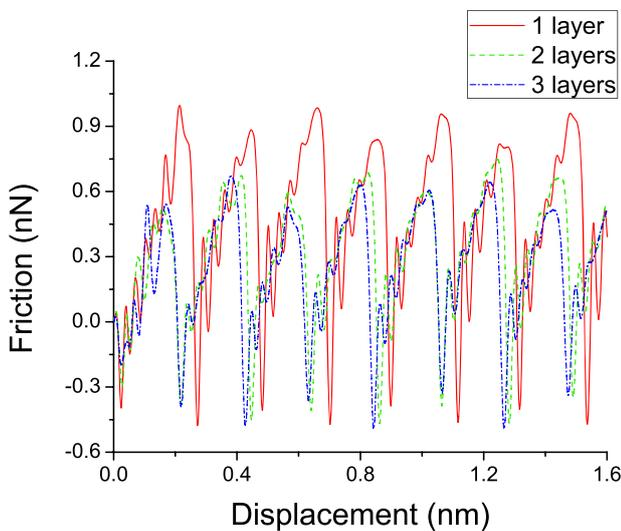
FIG. 2. Effect of number of graphene layers on friction for 42 nm long sheets.
