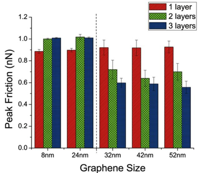
FIG. 3. The effect of graphene length on frictional layer-dependence.
