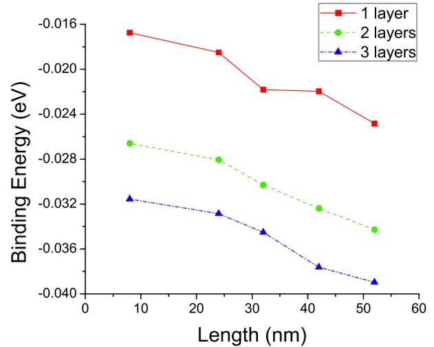
FIG. 6. Binding energy of multi-layer graphene decrease monotonically with sheet length.
