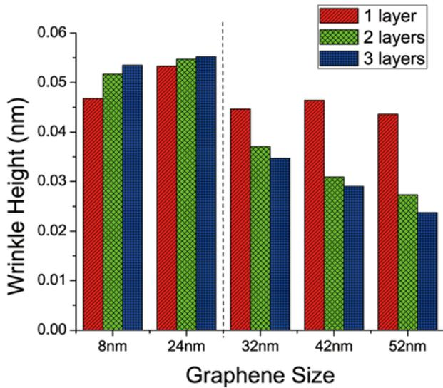
FIG. 5. Height of the wrinkle in front of the tip varying with number of graphene sheets and their length.
