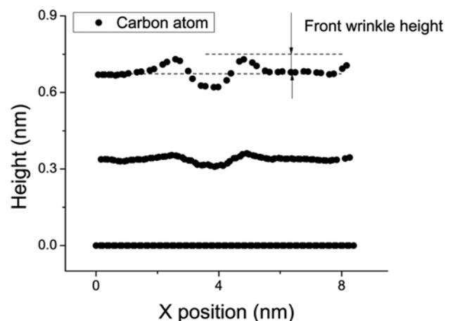
FIG. 4. Local profiles of the graphene layers during the scanning process.
