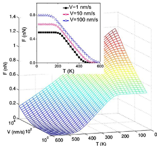
Fig. 4: (Colour on-line) Variation of the average friction with velocity and temperature with consideration of both thermal and instrument noise. The inset depicts the average friction as a function of temperature at different velocities.
