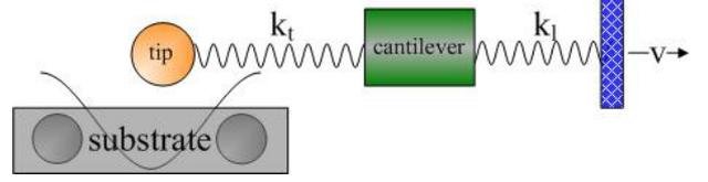
Fig. 2: (Colour on-line) Illustration of a two-spring, two-mass Prandtl-Tomlinson model. The support moving at a constant velocity drags the cantilever and the tip along the substrate.  $k_t$  and  $k_l$  are the tip and cantilever stiffness, respectively.
