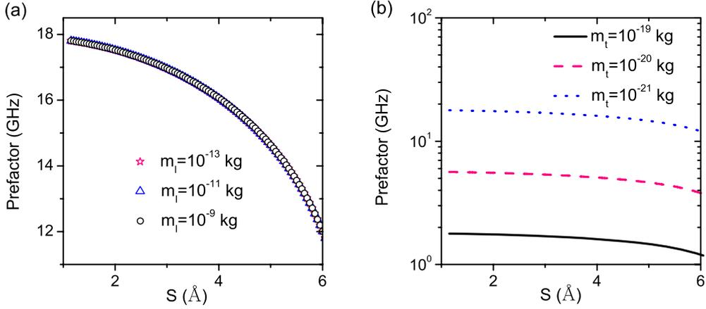
Fig. 3: (Colour on-line) Prefactor as a function of support displacement  $S$  demonstrating the effect of cantilever (a) and tip apex (b) masses. In (a) the tip apex mass is fixed at  $m_t = 10^{-21}$  kg, and in (b) the cantilever mass is fixed at  $m_l = 10^{-12}$  kg.
