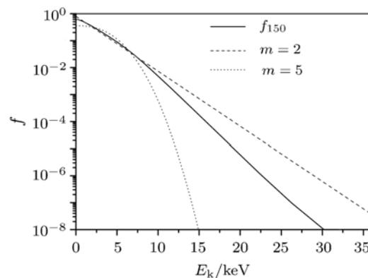
**Fig.4.** The simulated speed distribution function  $f(v)$  at  $x = 150$   $\mu\text{m}$ . Function  $f_{m=2}$  and  $f_{m=5}$  are also plotted for comparison.
