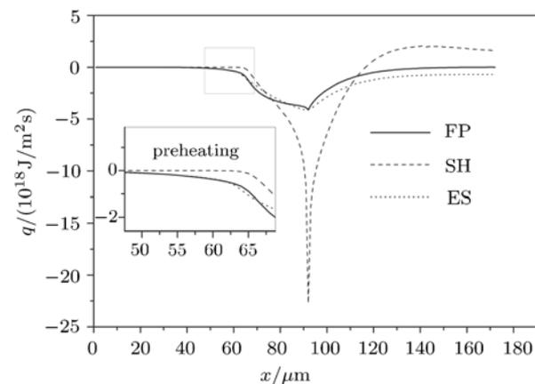
**Fig.2.** Comparison of the heat flux profiles obtained from Fokker–Planck result, SH result, and ES non-local result at  $t = 100$  ps and constant laser intensity  $I = 10^{14}$  W/cm<sup>2</sup>.
