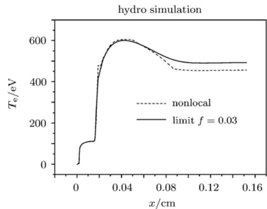
**Fig.6.** Hydro simulations using non-local model and flux limiting model, of temperature profiles after 1.5 ns irradiation with 351nm laser.
