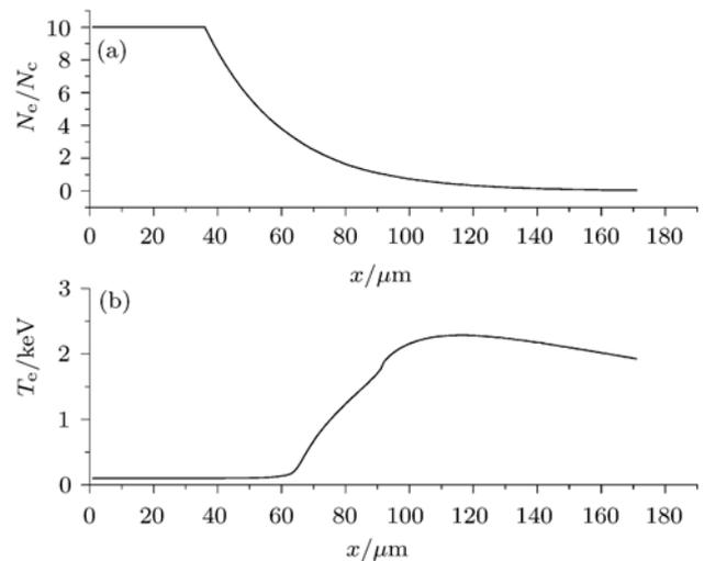
**Fig.1.** FP simulations of (a) electron number density(normalized to the critical density) and (b) temperature in keV, at the time  $t = 100$  ps.
