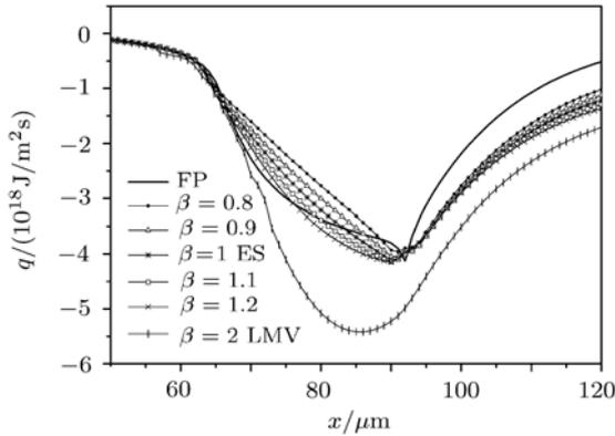
**Fig.5.** Comparison among heat flux profiles given by different  $\beta$  non-local models using FP simulation.
